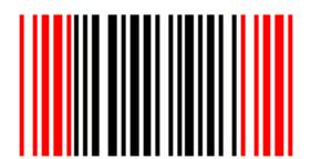
Code 39 is one of the oldest and most widespread bar codes in use. It uses the asterisk as its start and stop bar. Look for the same pattern of bars on the left and the right sides. The pattern is narrow bar, wide space, narrow bar, narrow space, wide bar, narrow space, wide bar, narrow bar.
